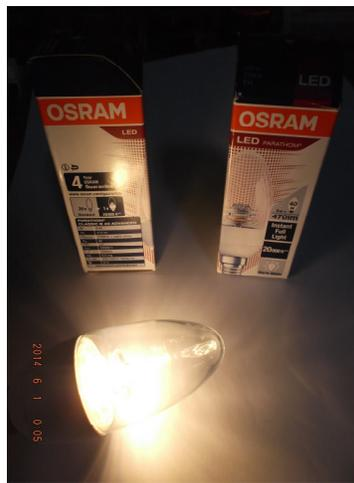
The difference between a quality dimmiable LED lamp with a wide flickerless dimming profile and a fast dimmer setting response, and a poorly operating one, can nearly always be traced back to the brand/ type of control chip inside the driver. The newer and more expensive chips have excellent dimming profiles, while the older chips are poorer and in some cases can hardly be considered dimmiable at all.
